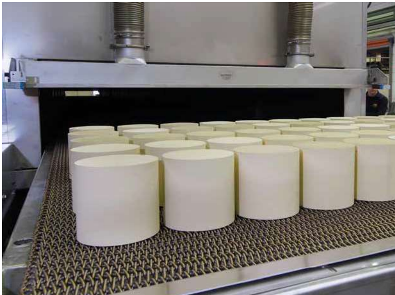
Fig. Ceramic honeycombs on oven belt
