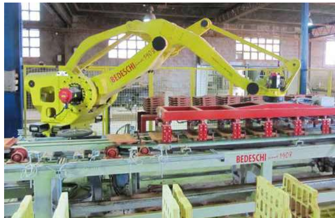
Fig. 2 Gripper for roofing tiles group re-forming
