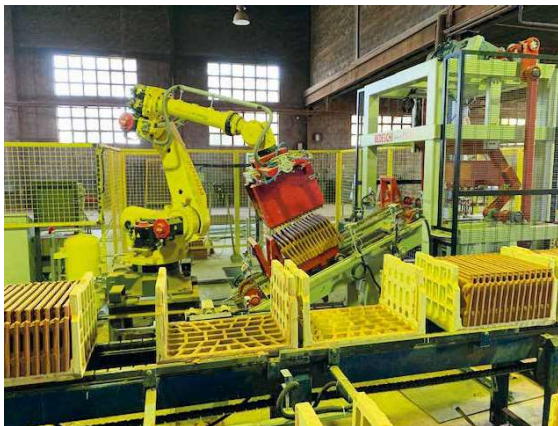
Fig. 1 Gripper for unloading roofing tiles into U-cassettes
