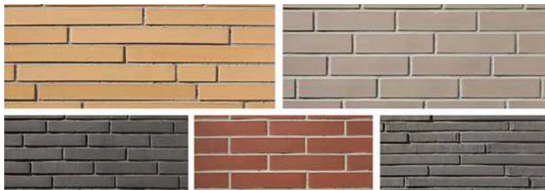
Fig. 1 Facing bricks decorated using the uniform coating method
