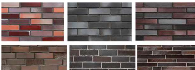
Fig. 2 Facing bricks decorated using the MULTICOLOR spraying system
