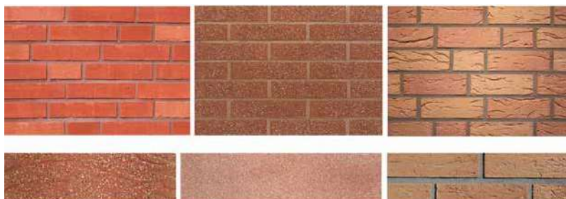
Fig. 4 Facing bricks decorated using sand application
