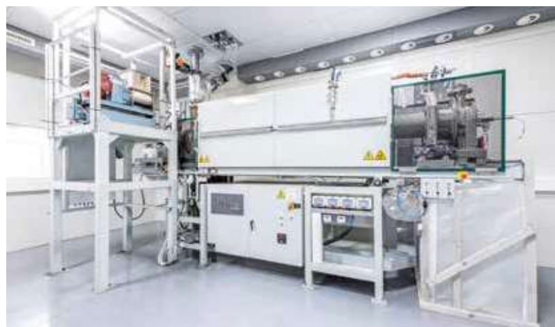
Fig. 2 Indirect rotary kiln IDO 7 at the IBU-tec Technical Center in Weimar
