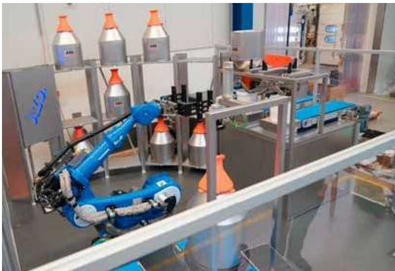
Fig. 3 AZO RoLog® – the robot for fully automatic charge supply and weighing of minor and small amounts of components
