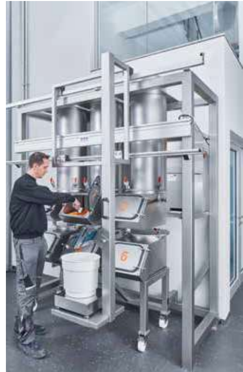
Fig. 4 AZO ManDos® – the operator-guided manual weighing station
