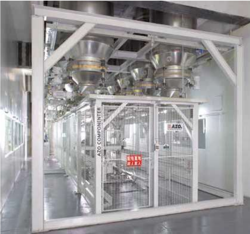
Fig. 2 AZO COMPONENTER® for the fully automatic weighing and charge supply of components
