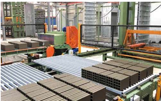
Fig. 6 Dryer car loading
