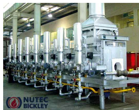
Fig. 10 Kiln with self-recuperative burners, capable of firing in flameless oxidation mode
