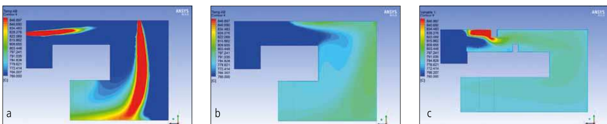
Fig. 6 a–c Temperature contours for three different designs of a thermal oxidizer
