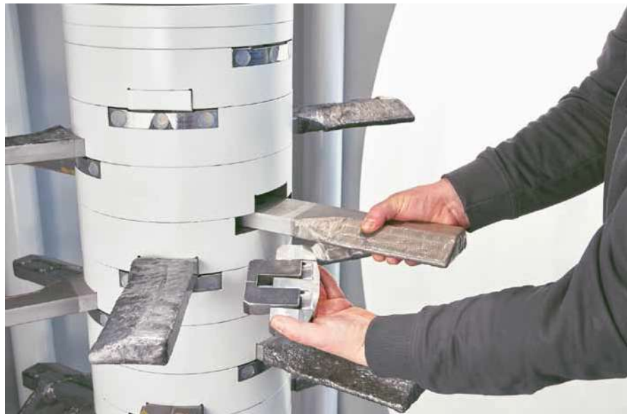
Fig. New SmartFix system – replacement of the beaters takes now only a few minutes (Source: Eirich)
