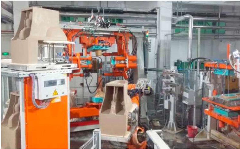
Fig. 2 View of the DORST Technologies WCM60 (center, background) and WRM60 (r.) high-pressure casting lines with handling robot (center, front) for the one-piece WC with concealed trap
