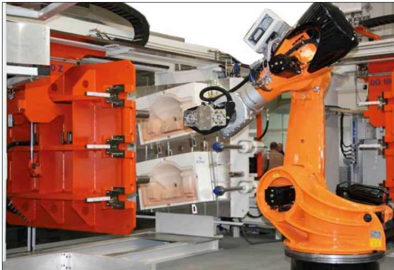
Fig. 1 DORST Technologies DG180 with two independent moulds and handling robot
