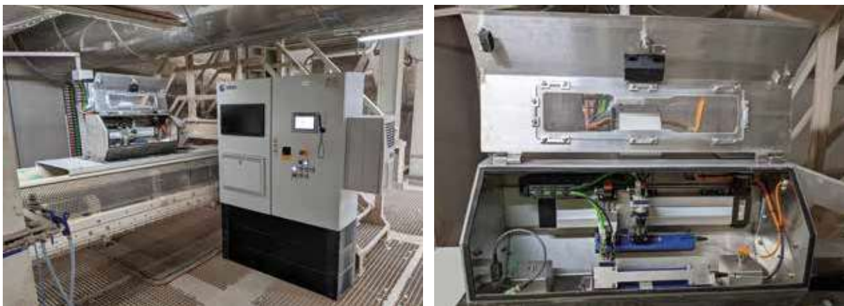
Figs. 1–2 Der Qualimaster VC1 for the optical quality assessment of granules
