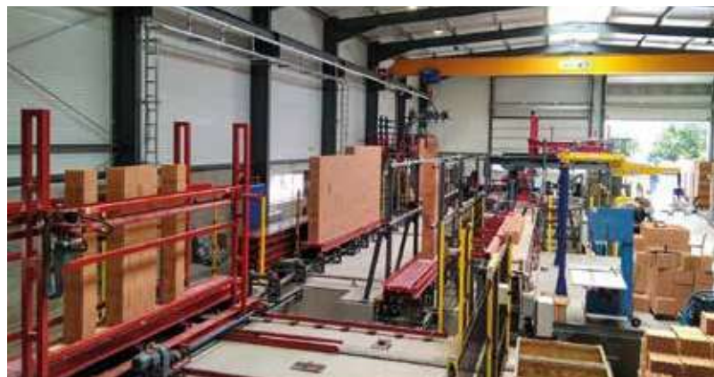
Fig. 2 Production of prefabricated wall elements
